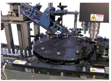
Chuck Capping Machines use a chuck head that is sized to a specific cap or range of caps, with some using a rubber chuck insert to help tighten caps onto the containers. Once the cap is in place, with manually or automatically, the chuck head descends to cover the cap and apply torque to create a consistent and reliable seal. Chuck cappers work with continuous thread closures such as flat caps, sports caps and more!
